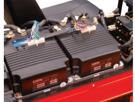
Curtis (USA) Electronic Controllers
