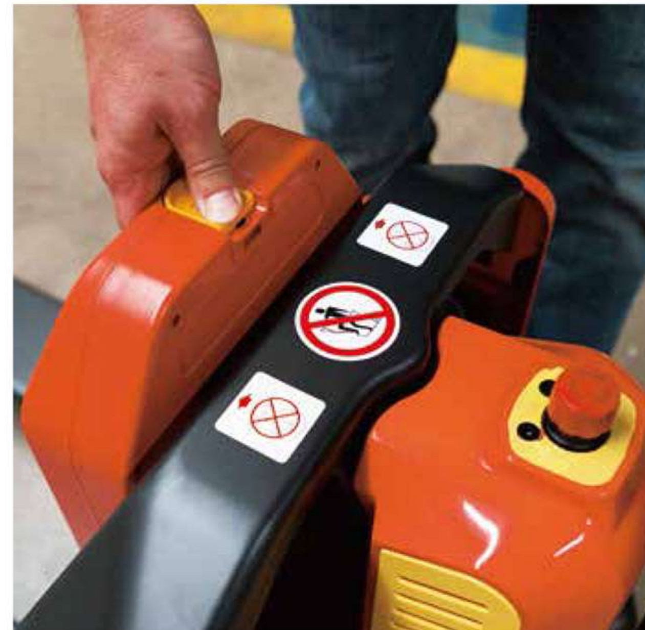
▲ Socket on battery case for easy battery charging without necessity to take the battery out
