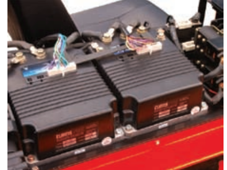
Curtis (USA) Electronic Controllers
