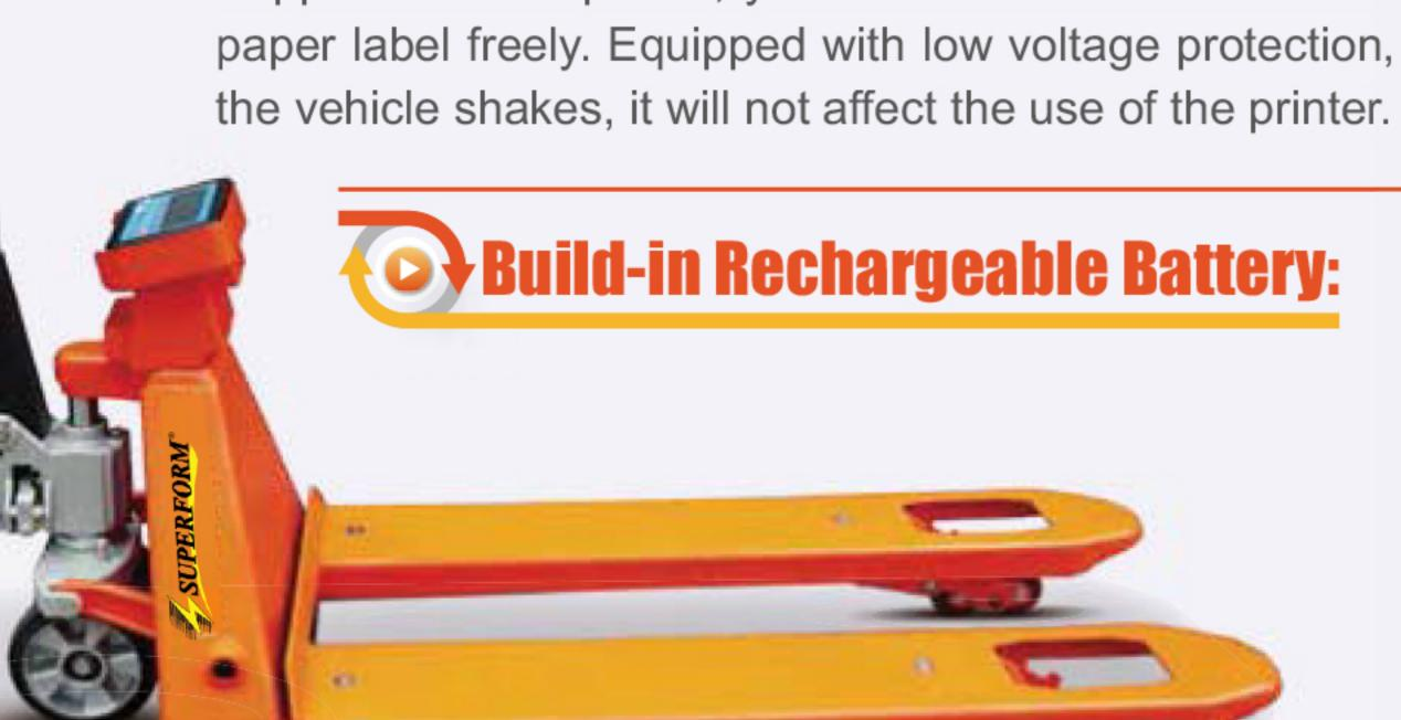
Built-in 4000mAH super-capacity rechargeable battery with the advantages of durability and convenient charging, without disassembly. It lasts 3 months on a single battery charge. and the operating current is only 1ma (on the premise that backlight and printer connection are turned off).
